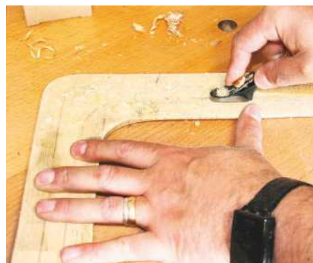
▲ Here the convex plane is ideal for contouring the underside of a boomerang
